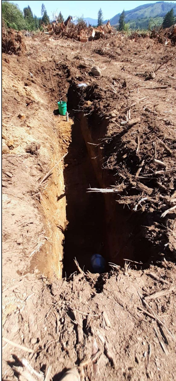
Conducting Infiltration Testing, TP-5
