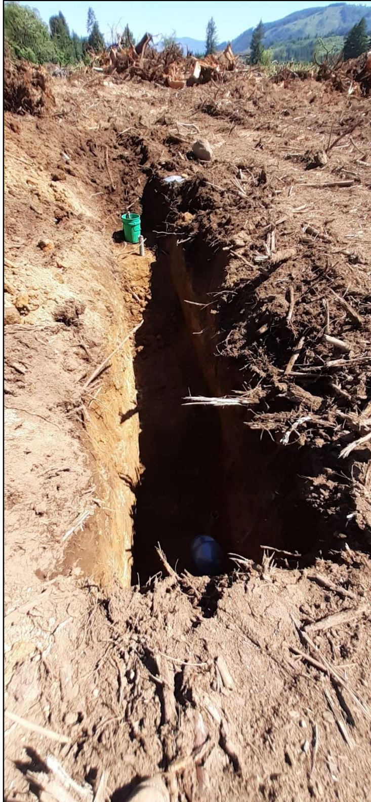
Conducting Infiltration Testing, TP-5
