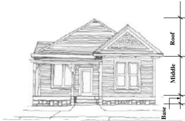
FIGURE 6-4 EXPRESSION OF BASE, MIDDLE AND ROOF ELEMENTS
