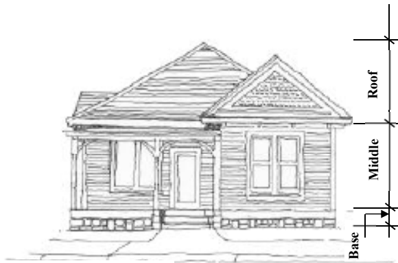
FIGURE 6-4 EXPRESSION OF BASE, MIDDLE AND ROOF ELEMENTS
