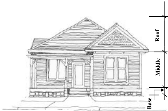
FIGURE 6-4 EXPRESSION OF BASE, MIDDLE AND ROOF ELEMENTS
