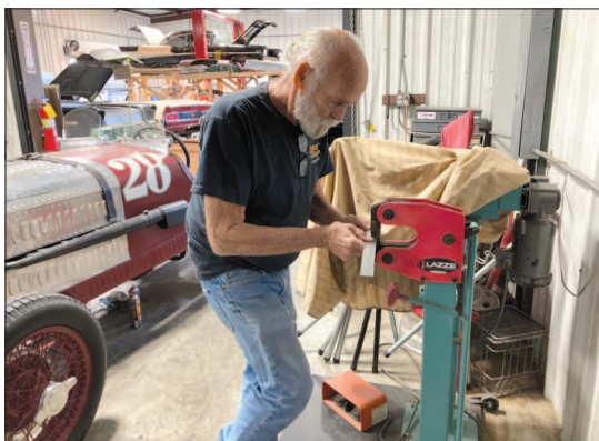
Sachse Rod Shop owner bends a piece of metal using a machine called a shrinker stretcher. Millsap said since the onset of the pandemic, his shop has had issues getting parts. Millsap is able to make some parts need in his shop, which gives him a slight advantage.
