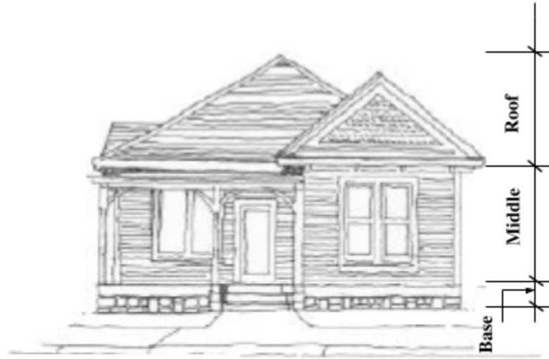
FIGURE 6-4 EXPRESSION OF BASE, MIDDLE AND ROOF ELEMENTS
