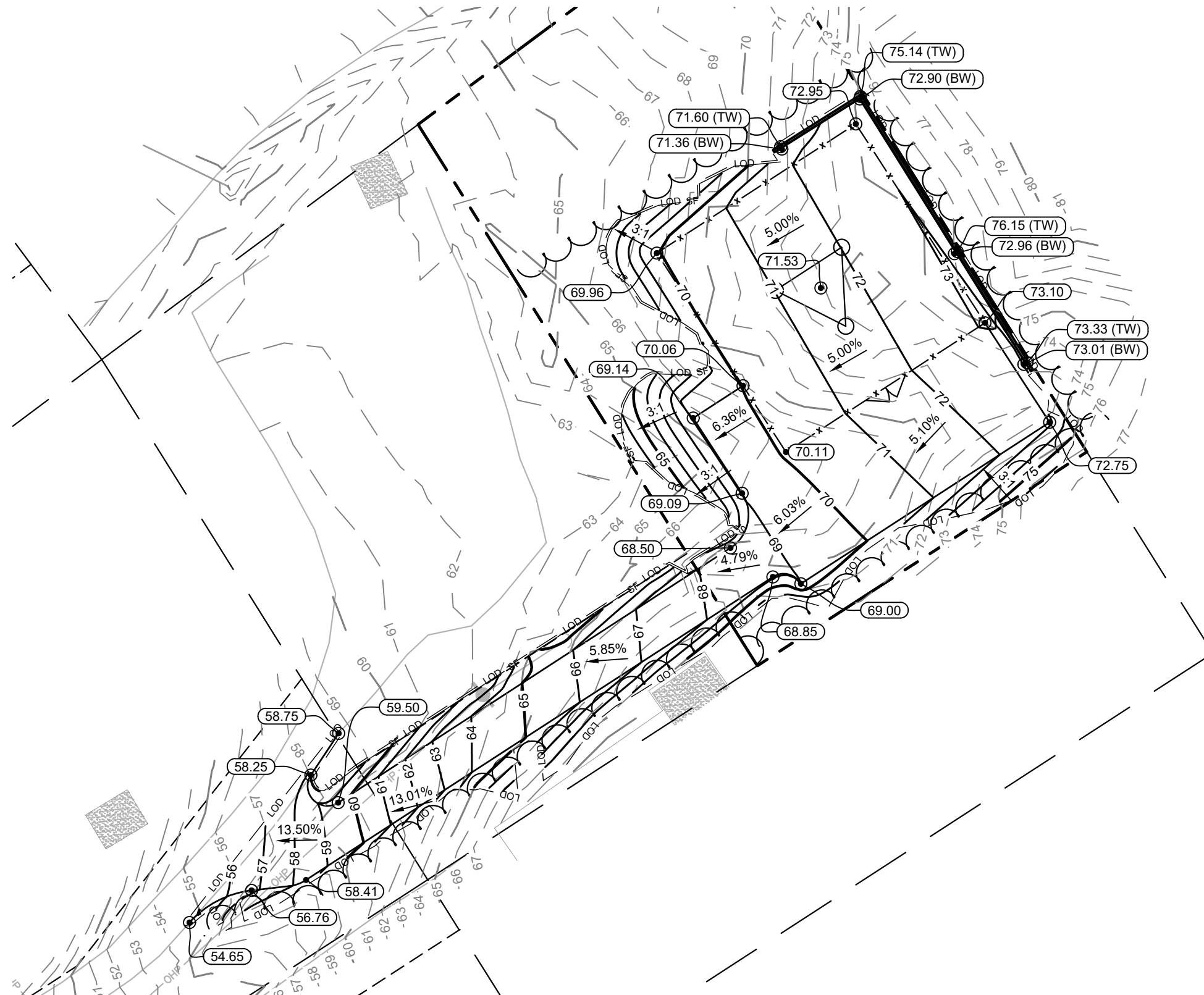
1 GRADING AND EROSION CONTROL PLAN C8 SCALE: 1" = 30'
