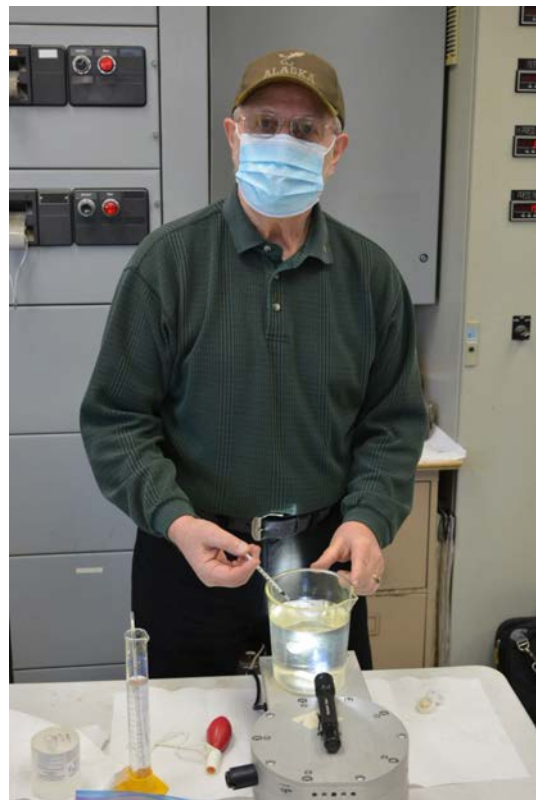
27) Mike Pollen performed jar tests of the raw water using the same type of coagulant that was used in the DAF pilot tests run in 2016. This was the first time the DAF process chemistry had been tested under late winter water quality conditions from the Wrangell source water. UVA 254 and UVT tests were run on filtered samples to measure organic matter removal in the tests.
