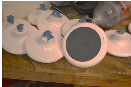
10) Ozone is diffused into the raw water through ceramic diffusers. These are new ones to replace the older diffusers which scaled up.
