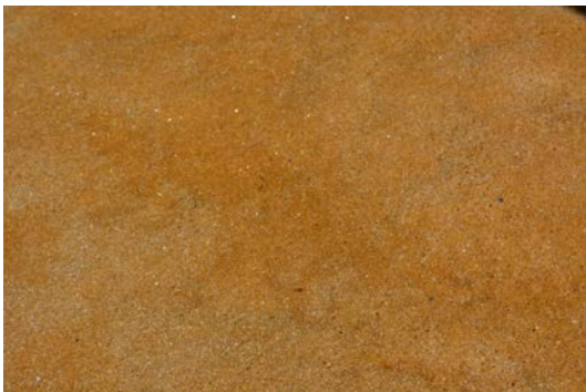
20) Iron fouling is evident on the otherwise grey filter sand media. This is the surface of filter #4 after draining. There was no visible evidence of a dark biofilm layer (schmutzdecke).
