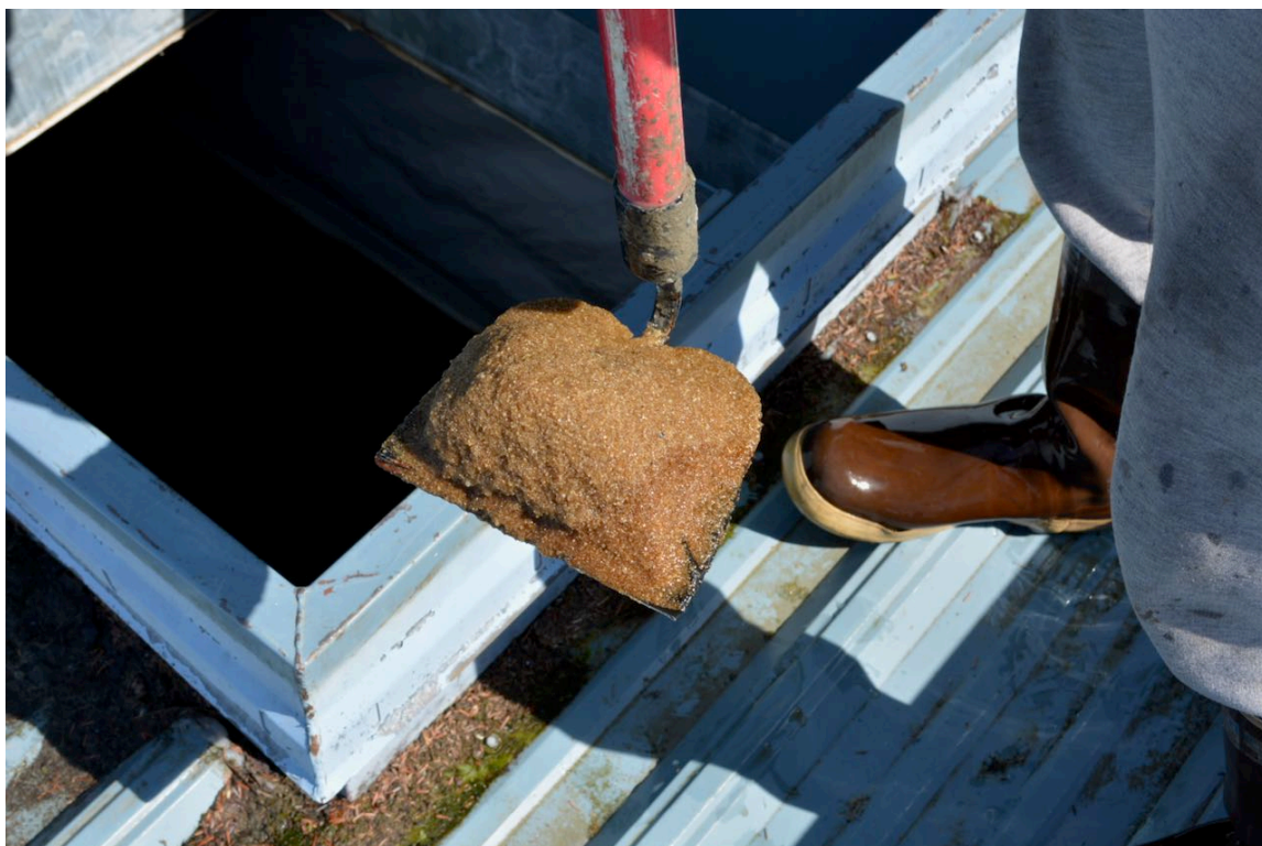
Figure 4: Wayne McHolland holds the sample skimmed from the surface of Slow Sand Filter #4 with a garden hoe on April 5. Iron has discolored the sand and no biofilm (“Schmutzdecke”) was visible on the surface of the sand.
