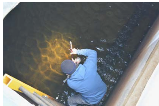
17) On April 14, Wayne McHolland collected samples from the surface of slow sand filters #2 and #4. These were transported back to Fairbanks where Mike Pollen examined them with 100x, 200x, 400x, and 1,000x light and phase contrast microscopy.
