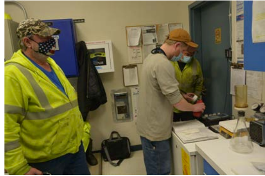
26) CBW water system operators calibrate the pH meter during the process monitoring class.
