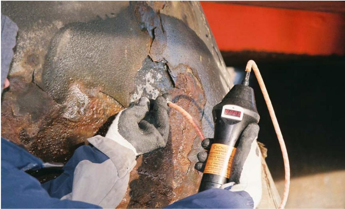
**PHOTO No. 5:** Southern Floatation Tank Pipe Strut – Note the coating failure and corrosive scale evident in the splash zone. Level III ultrasonic thickness measurements found the remaining thickness to be 0.357 inches.
