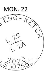
**RECOVERED 5/8" REBAR** WITH 2" ALUMINUM CAP. IN GOOD CONDITION
