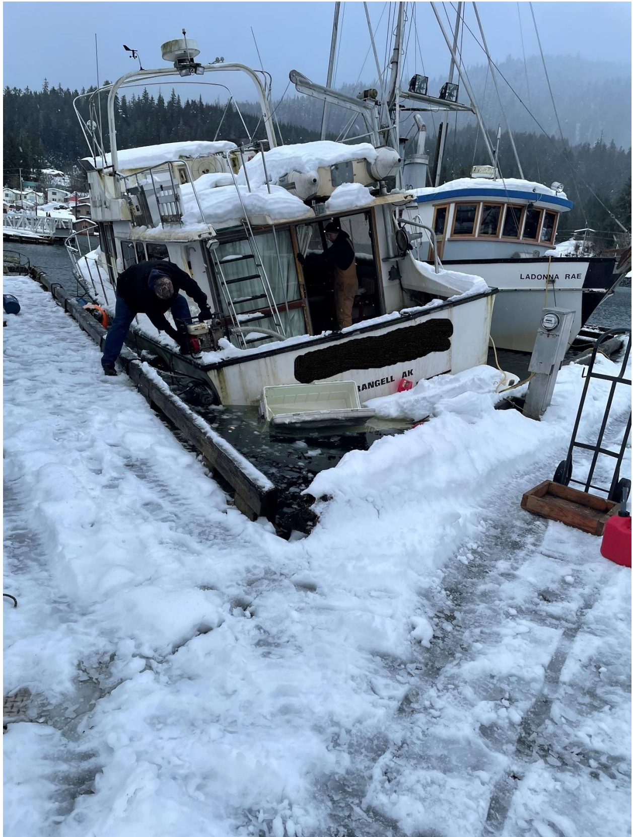
Sea Chest frozen and wet heavy snow overload.
