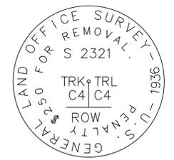
RECOVERED 2.5" DIA. BRASS CAP ON A 1" X 30" STEEL PIPE MONUMENT. IN GOOD CONDITION
