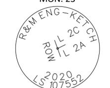
RECOVERED 5/8" REBAR WITH 2" ALUMINUM CAP. IN GOOD CONDITION
