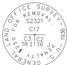
RECOVERED 2.5" DIA. BRASS CAP ON A 1" X 30" STEEL PIPE MONUMENT. IN GOOD CONDITION
