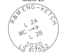
RECOVERED 5/8" REBAR WITH 2" ALUMINUM CAP. IN GOOD CONDITION
