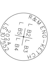
SET 5/8" X 30" LONG REBAR (UNLESS OTHERWISE NOTED) AND 2" ALUMINUM CAP WITH PLASTIC INSERT
