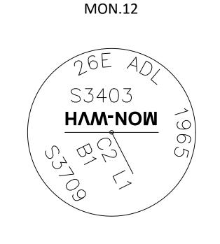
RECOVERED 2.5" DIA. BRASS CAP ON A 2" STEEL PIPE MONUMENT PROJECTING 11" ABOVE GROUND. IN GOOD CONDITION
