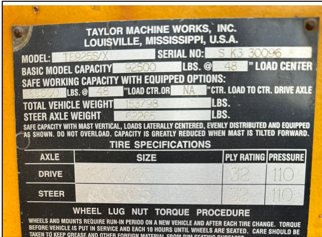
FIGURE 19. Data plate on forklift with weight and lifting capacity.
