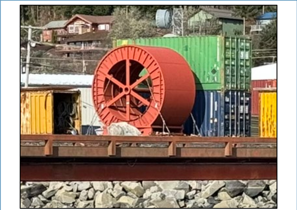
FIGURE 21. Steel electrical cable spool; weight estimated to be over 40 tons.
