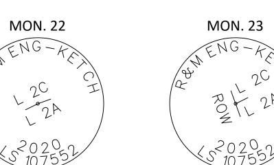
**RECOVERED 5/8" REBAR** WITH 2" ALUMINUM CAP. IN GOOD CONDITION
