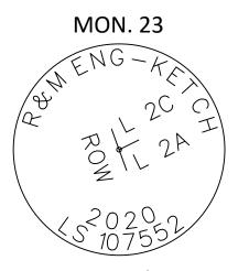
RECOVERED 5/8" REBAR WITH 2" ALUMINUM CAP. IN GOOD CONDITION
