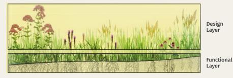
In this **layered planting** there is density above and below ground. The underground root layer can play an important role in managing stormwater runoff.
