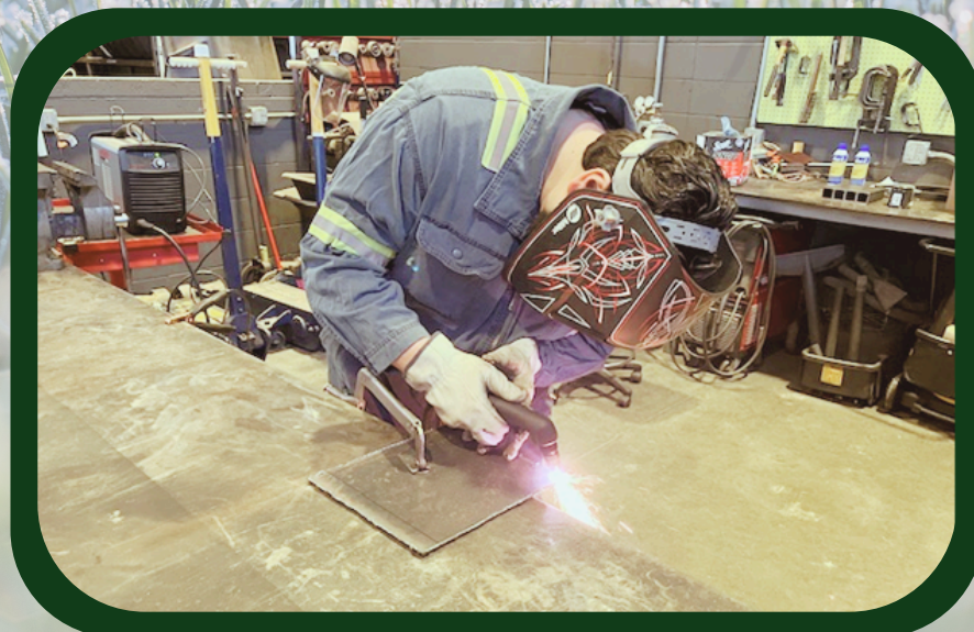
Fleet Mechanic Jose Mora, cutting bases for new brackets
