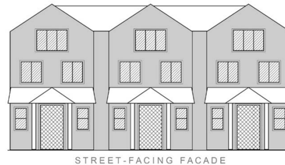
STREET-FACING FACADE ■ Area subject to 15% window & entrance door coverage requirement ▨ Qualifying window coverage ▩ Qualifying entrance door coverage
