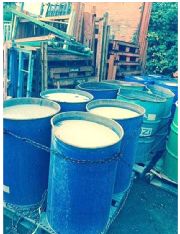
Improperly stored process water
