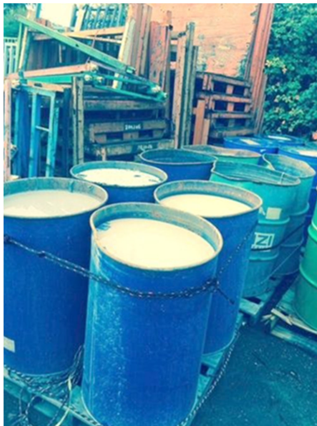
Improperly stored process water
