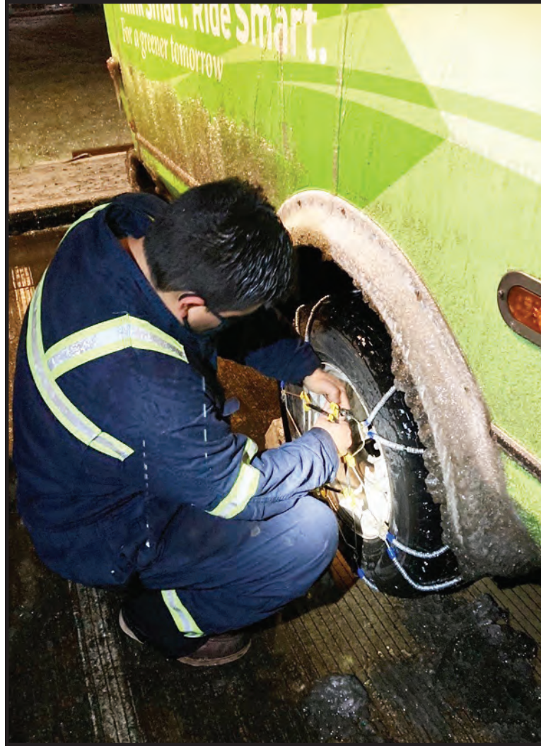
Fleet staff installing chains on SMART bus during inclement weather.
