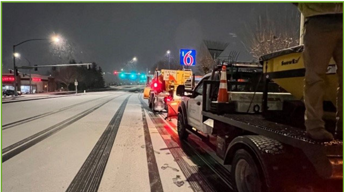
Sanding equipment on Elligsen Road
