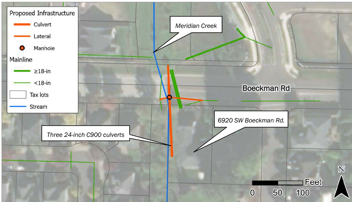
Figure X-X. Meridian Creek Culvert Replacement
