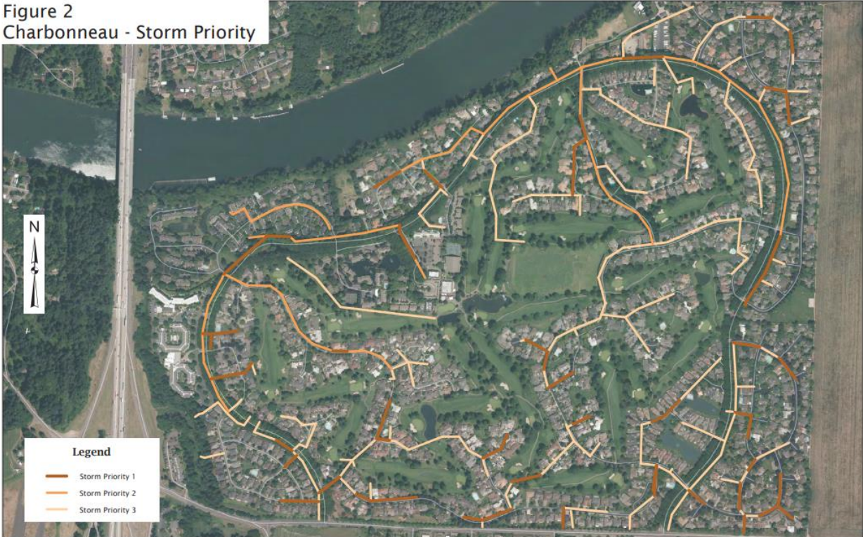
Stormwater replacement prioritization from Charbonneau Consolidated Improvement Plan (2014)
