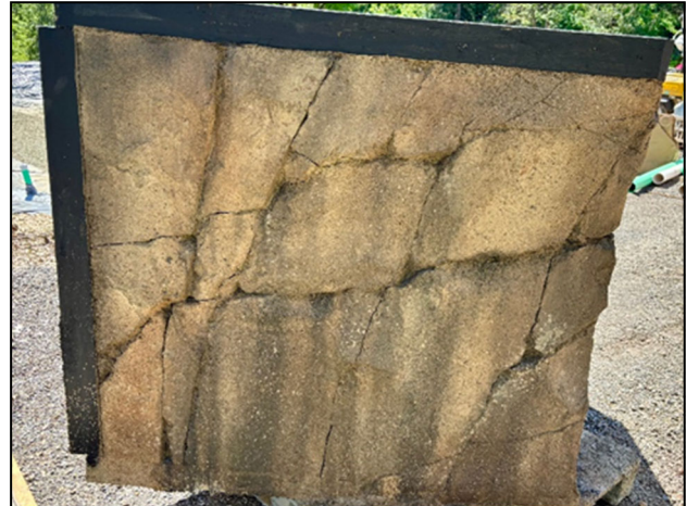
A shotcrete "rock face" wall is being installed at the east side of the trail under the bridge (left). The shotcrete is hand carved to resemble a rock face (right). The test panel is 6 feet tall.
