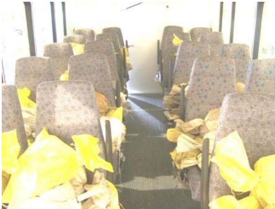
BUS LOADED TO 2.5 TIMES GVL (7,875 LBS)
