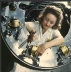
Part of the cowling for one of the motors for a B-25 bomber is assembled in the engine department of North American [Aviation, Inc.]'s Inglewood, Calif., plant (Library of Congress) https://www.loc.gov/item/2017878516/
