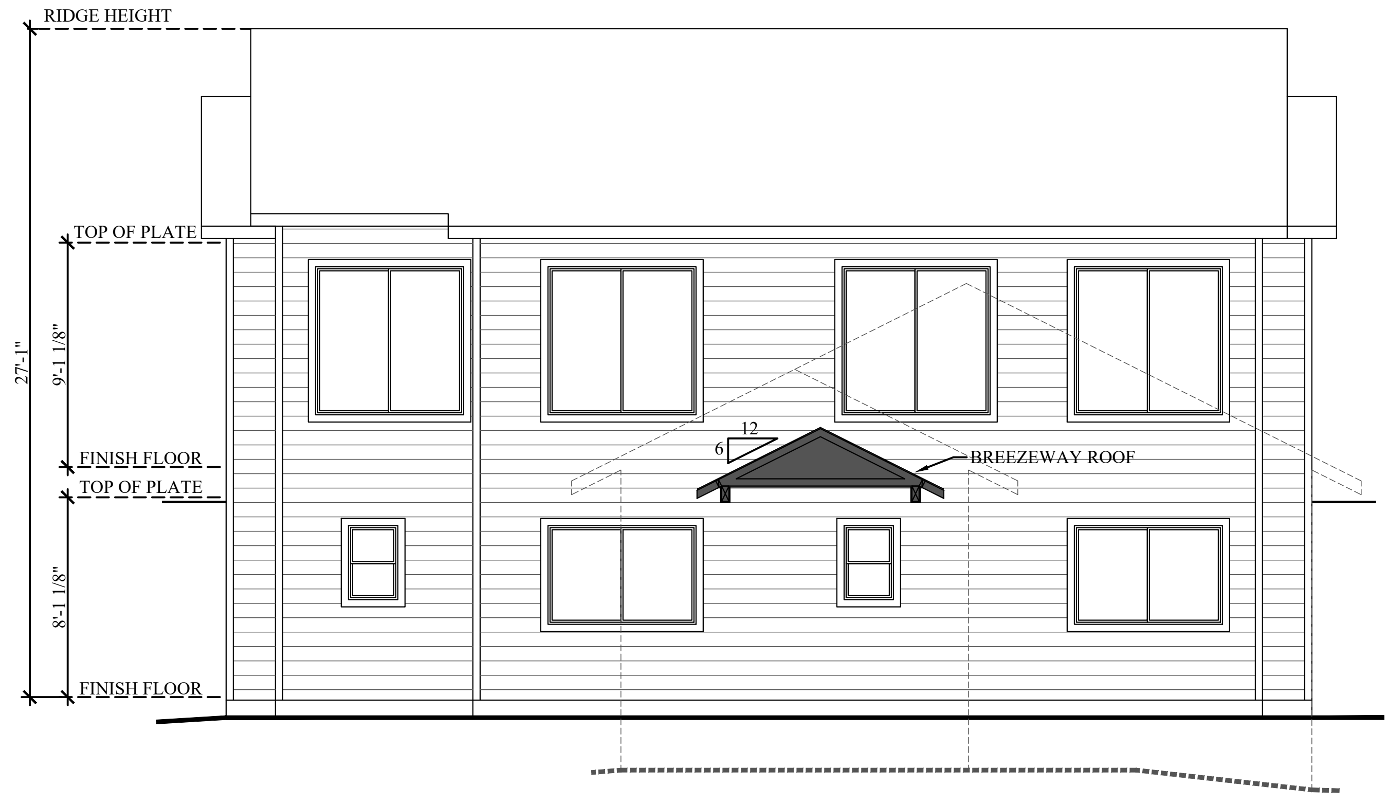
UNIT A & B REAR ELEVATION 1/4" = 1'-0"
