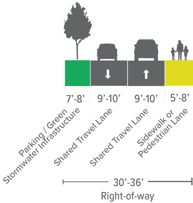
Figure 29 Cross-Section for Constrained Neighborhood Street
