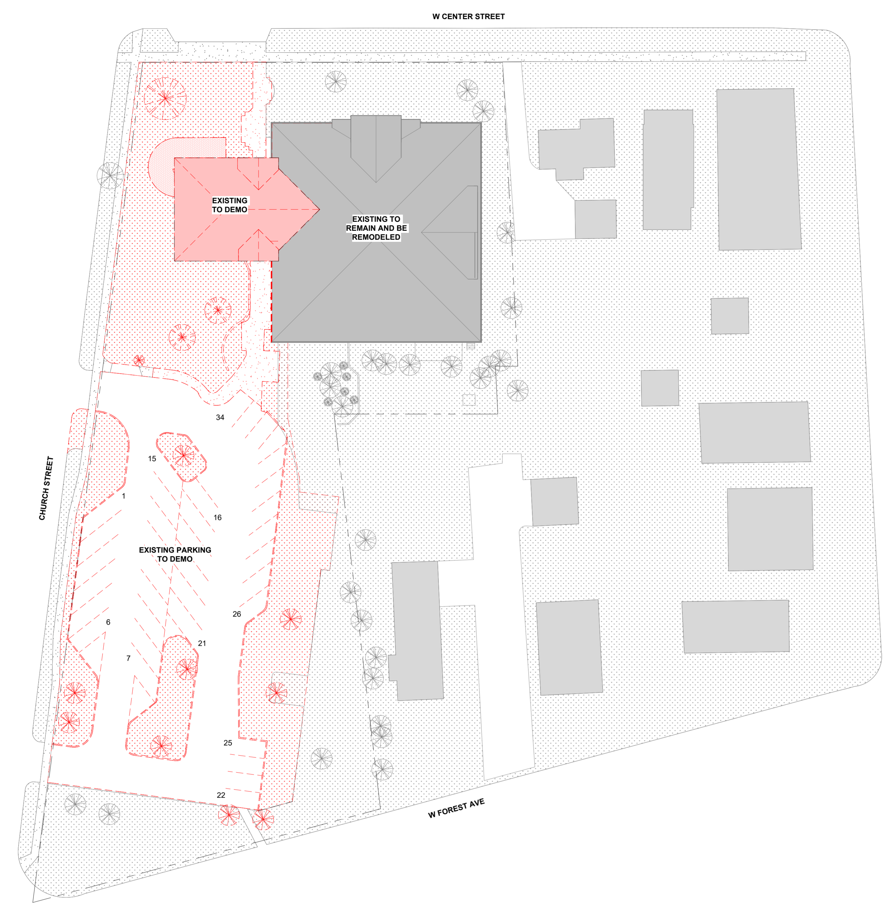
1 Architectural Site Plan - Demolition 1" = 30'-0"
