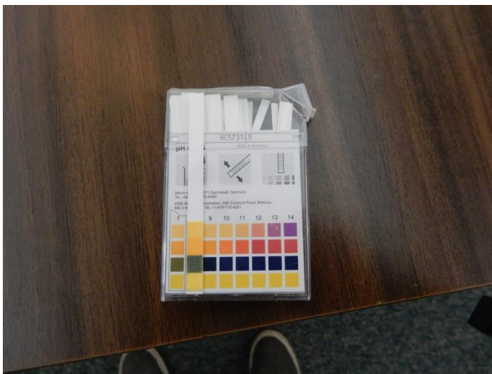
Image 13: Example of pH Test Strips
