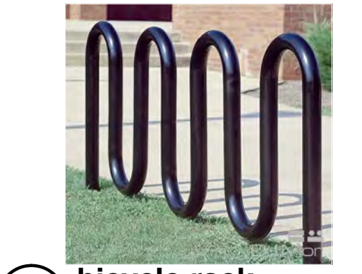
5I bicycle rack (1-CONDITION) BIKE RACK BY DUMOR INC. MODEL NO. 130-20 (8-2 SURFACE PLATE MOUNT) 2 3/8" O.D. BLACK POWDER-COATED LOOP OR EQUAL
