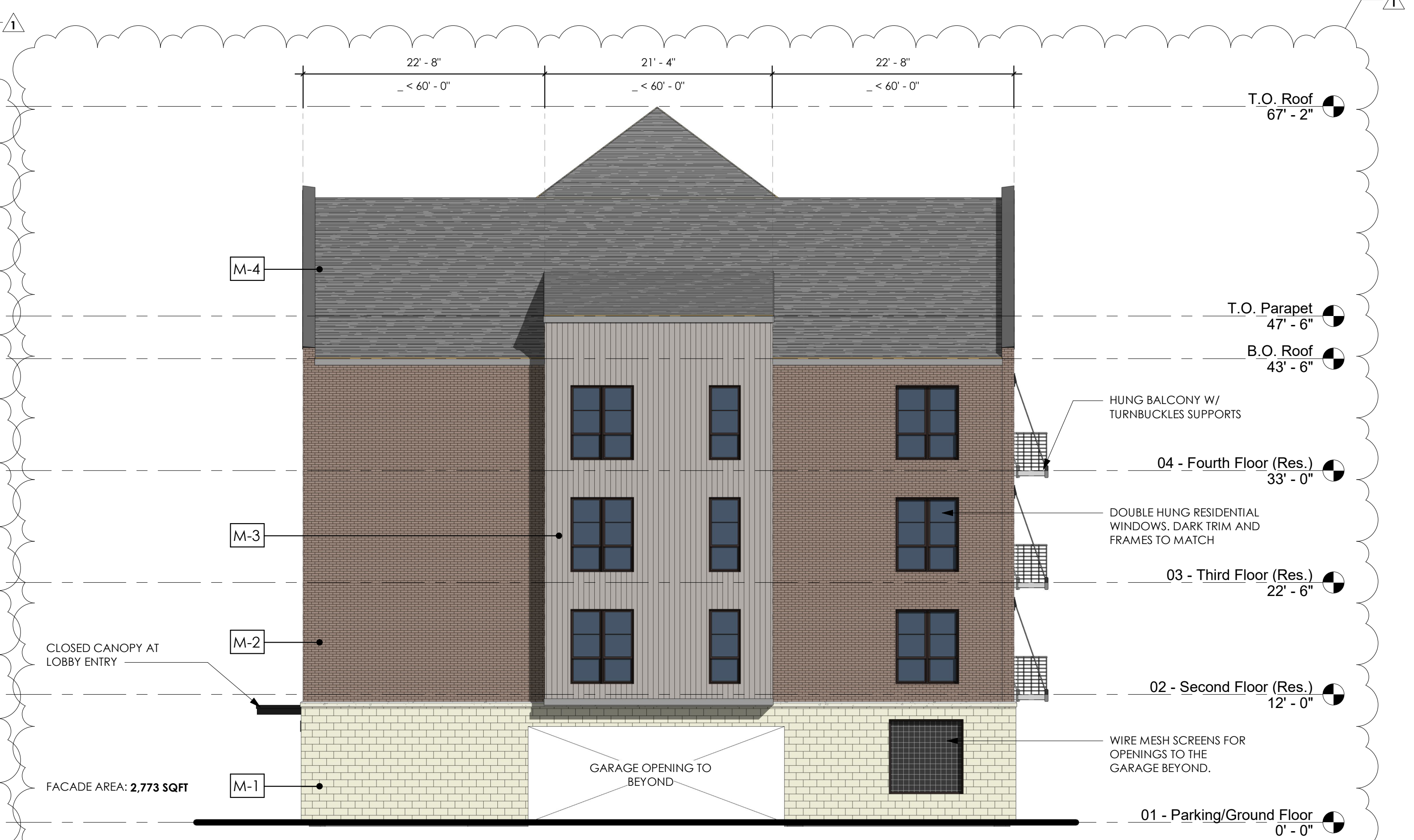
Side Elevation (Vehicle Entry)
