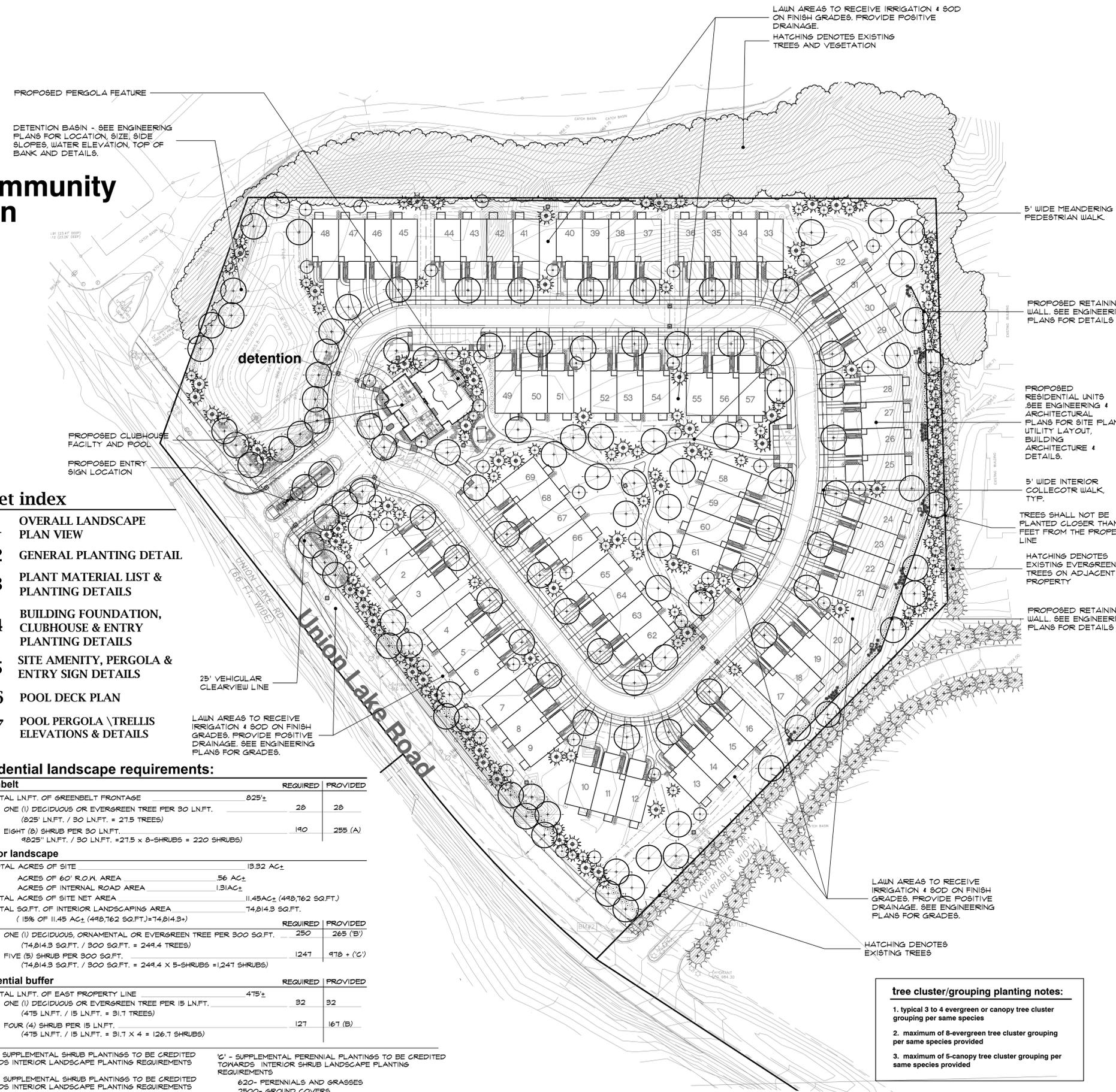
LAWN AREAS TO RECEIVE IRRIGATION & SOD ON FINISH GRADES. PROVIDE POSITIVE DRAINAGE.
