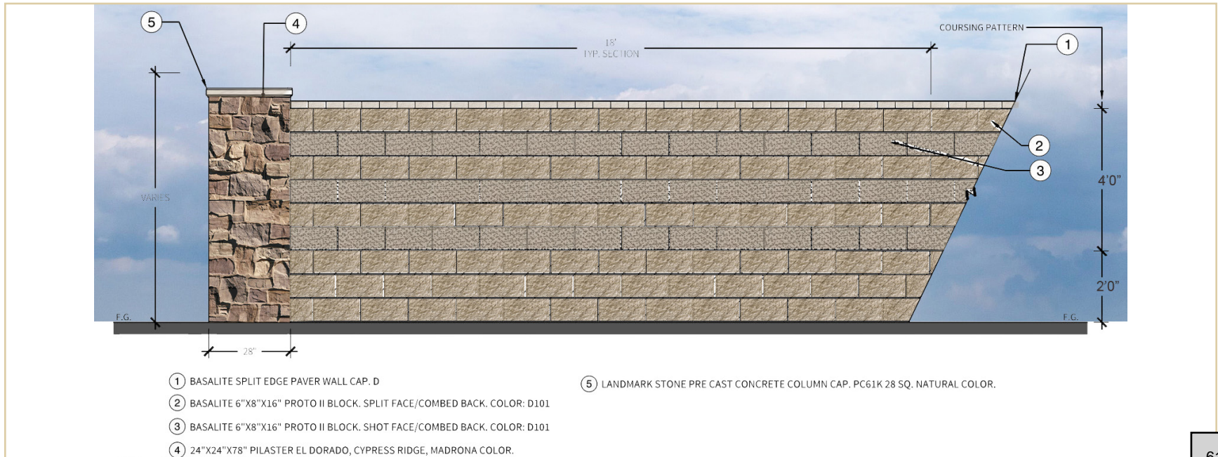
FIGURE 5A: Masonry Wall
