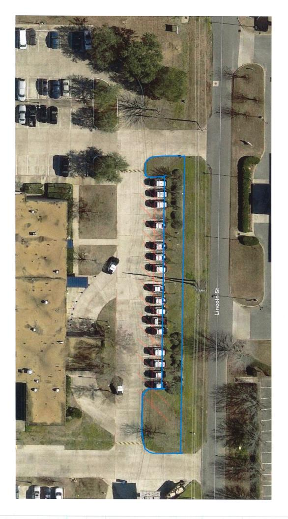
The area outlined in blue will be the extent of the new 8,700 sq ft of 5" thickness concrete paved area. The light red lines show the approximate striping for the 40 newly created parking spaces. Each space will also have a concrete parking bumper.
