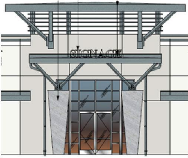
Figure 6-7: Ground Floor Permanent Canopy Sign
