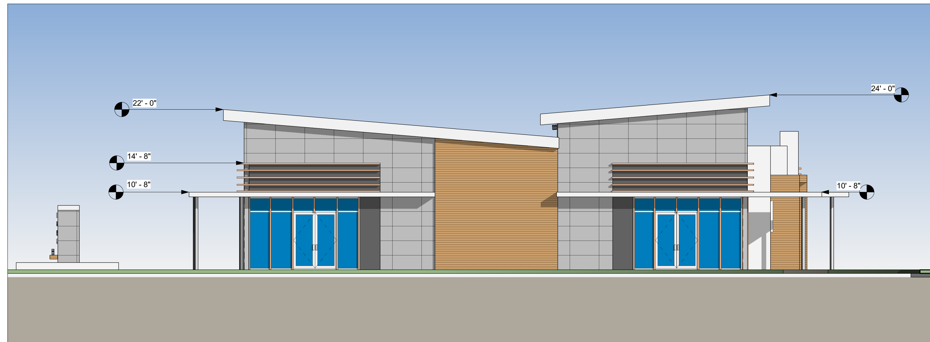
1 A3.02 EXTERIOR ELEVATION - NORTH 1/8" = 1'-0"
