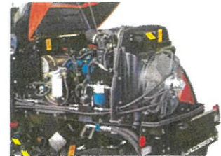
Trustworthy Kubota® engine & cooling reversing fan
