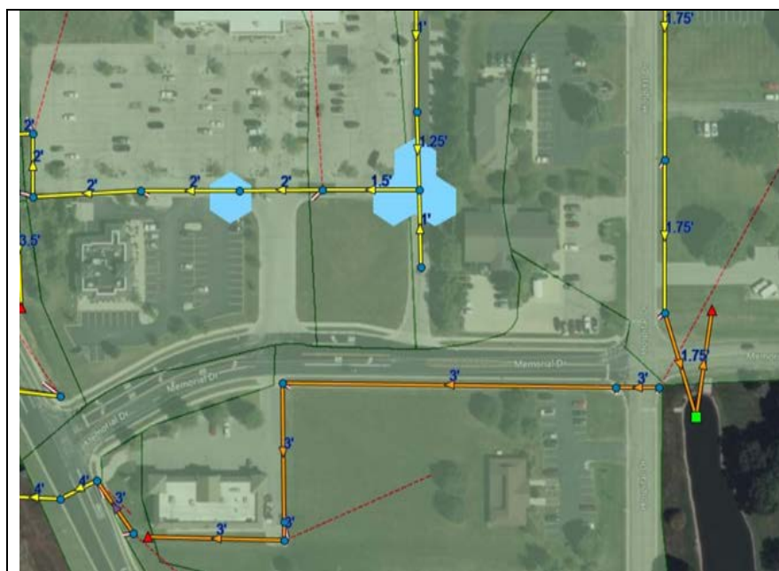
Figure 2. Flooding conditions after implementation of recommendations during the 100-year event at the intersection. The locations of proposed pipe upsizing are in orange. The proposed wet-detention basin is represented by a light green box. Approximately 1,200 lineal feet of 21 to 36-inch storm sewer will be provided as part of the proposed upsizing.
