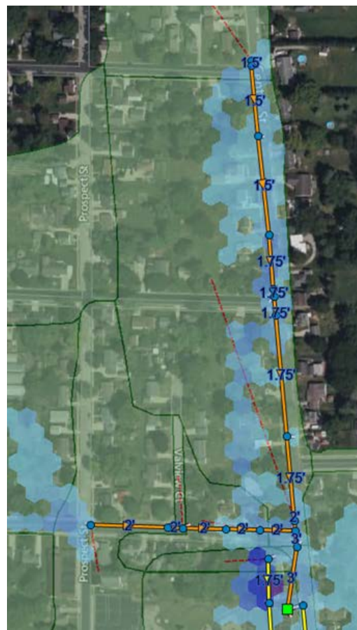
Figure 1. Existing flooding conditions in SSL1.3 during the 100-year storm event.
