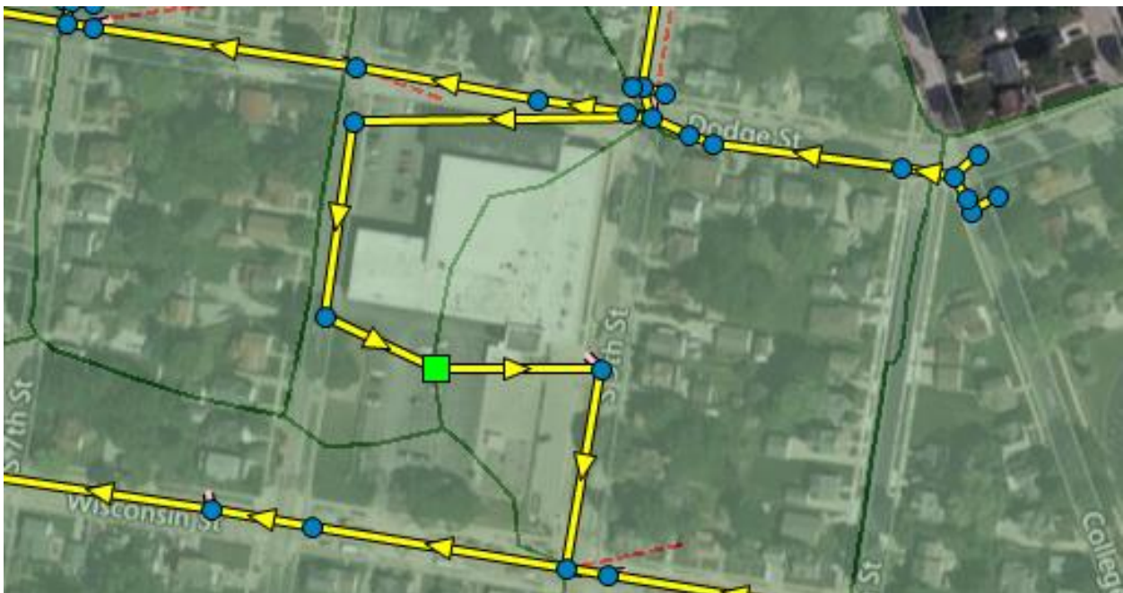
Figure 3. Proposed underground storage location and proposed storm sewer routing adjustment.
