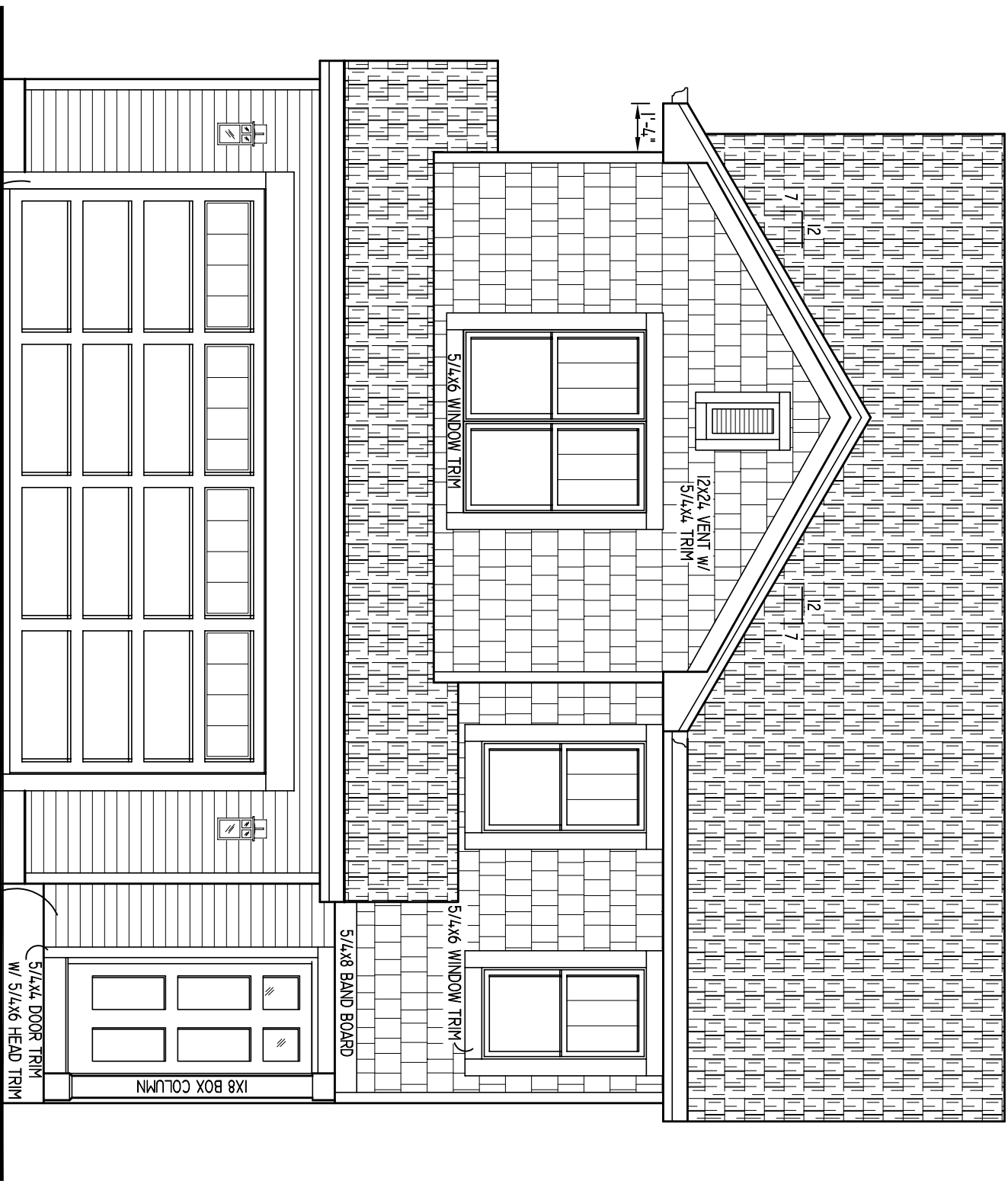
FRONT ELEVATION SCALE: 1/4" = 1'-0"
