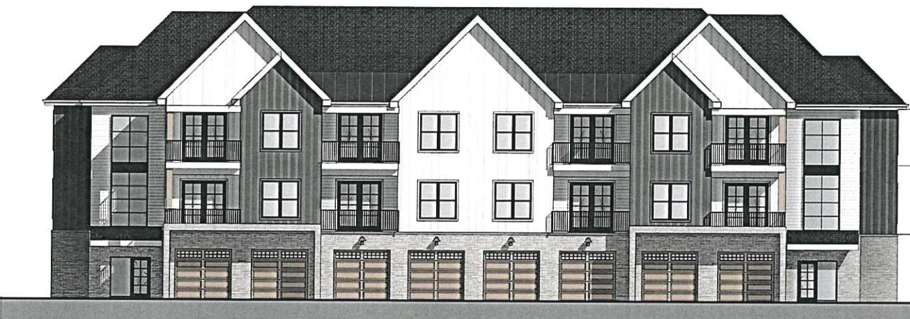
③ BUILDING C - FRONT ELEVATION 1/16" = 1'-0"
