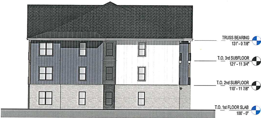
1 BUILDING A - RIGHT SIDE ELEVATION 1/8" = 1'-0"
