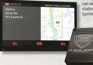
In Dispatch Centers and administrative areas, the HDTV Remote can be used to display a list of recent alerts with individual station success indicators, (optional) incident map locations, system and radio channel status, and Station Controller alarms.
