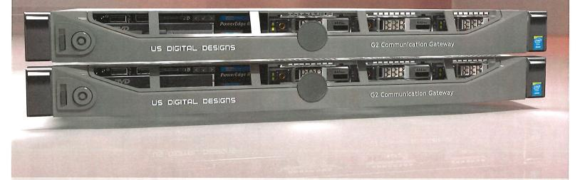
The G2 Communications Gateway is the link between the CAD system at the dispatch center and the G2 ATX Station Controller hosted at each fire station.
