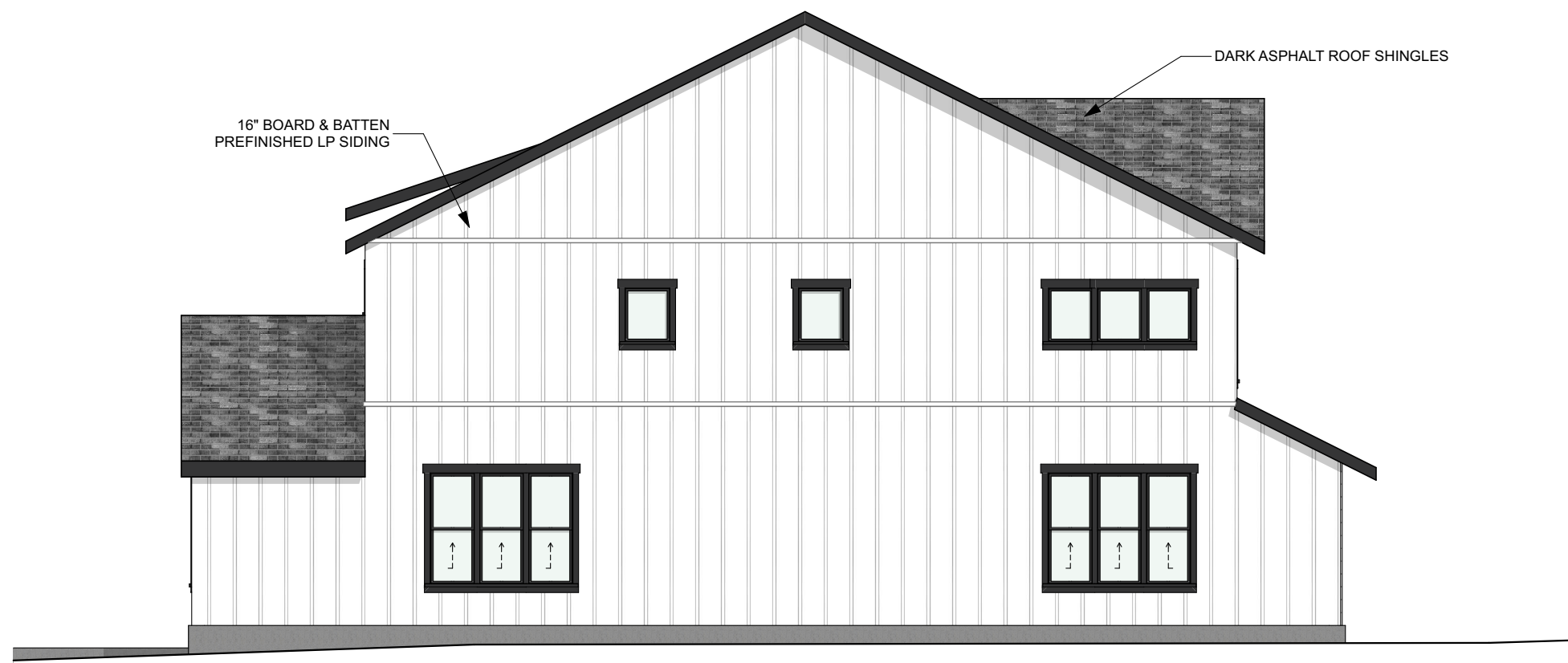
2 SOUTH ELEVATION BUILDING A SD202 SCALE: 1/8" = 1'-0"
