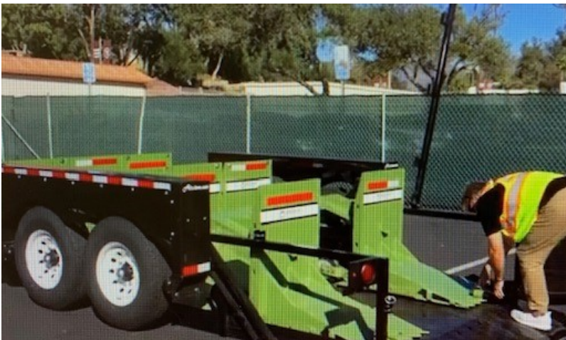
3. Barrier system on trailer.
