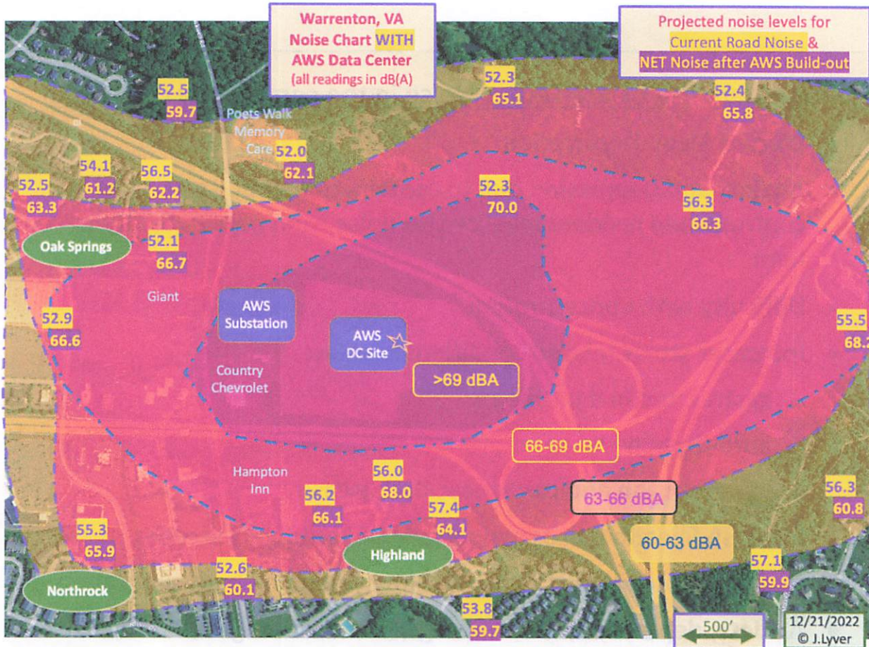
Predicted Exceedance of the ToW Noise Ordinance Limits at the Parcel Boundary
