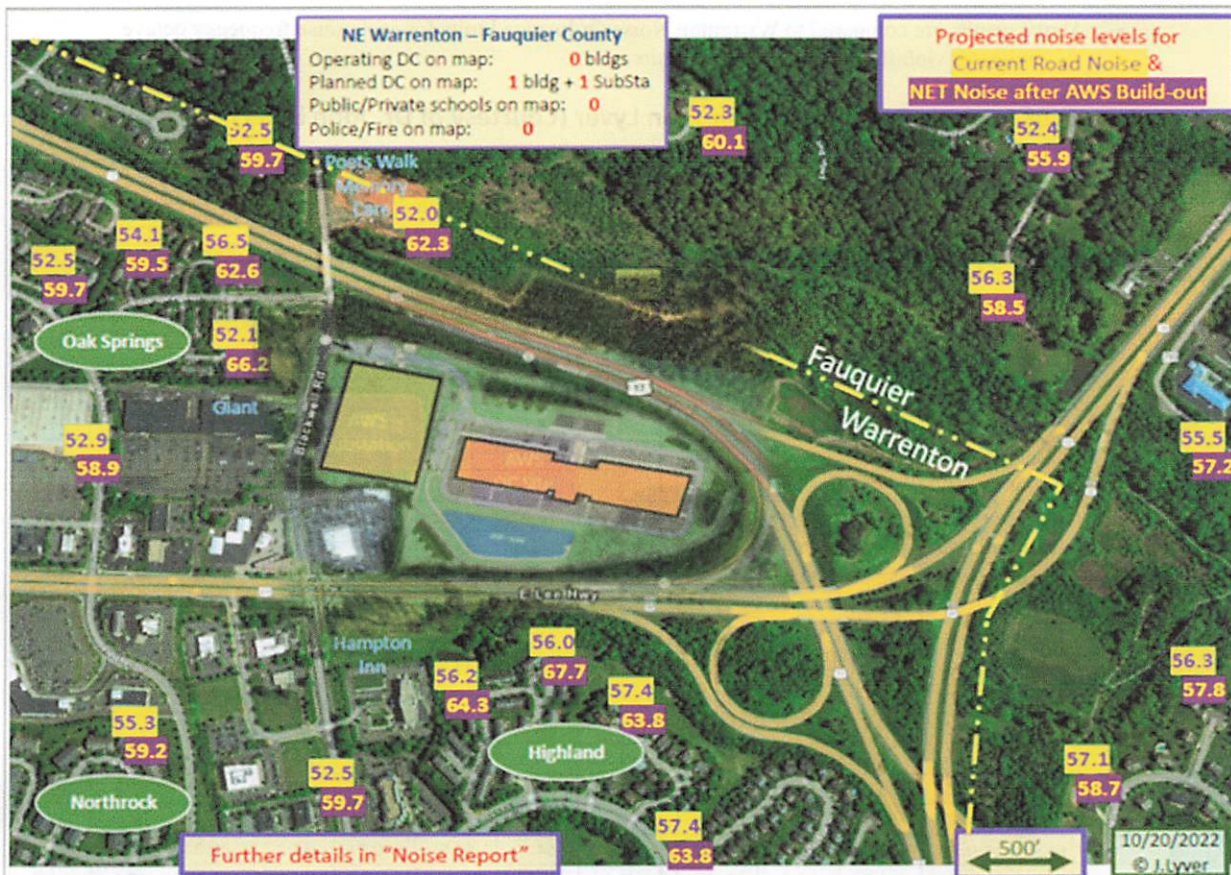
Figure identifies 21 locations within 2500 feet of proposed AWS location where noise has been modeled. Noise emissions were modeled on several similarly sized and recently built AWS facilities in Prince William County. Yellow tabs identify ambient traffic noise and purple tabs identify expected post-construction operating noise levels. Both are measured in dBA scales.
