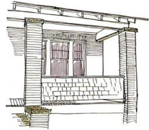
Brick Pier with Concrete Capping and pannel railing
