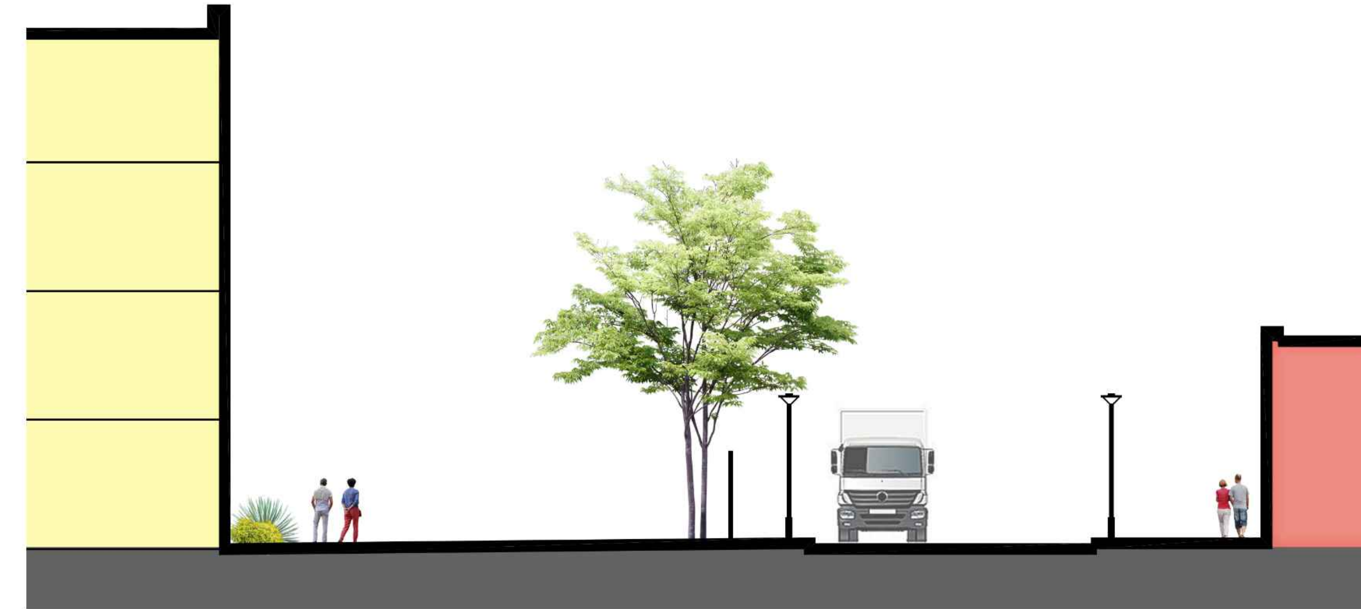
GREEN BUFFER (VARIES) BETWEEN RESIDENTIAL AND ALLEY ALLEY SIDEWALK / RETAIL LOADING + TRASH ZONE (VARIES)
