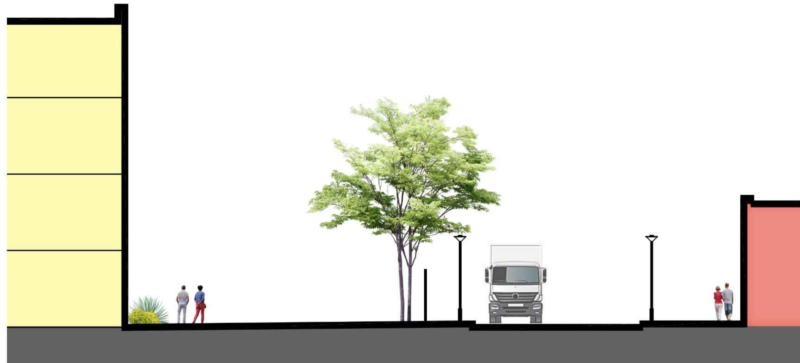
GREEN BUFFER (VARIES) BETWEEN RESIDENTIAL AND ALLEY ALLEY SIDEWALK / RETAIL LOADING + TRASH ZONE (VARIES) TYPICAL SECTION THROUGH ALLEY SCALE 1/8"=1'-0"
