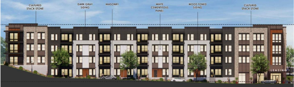
Block 1 Multi-Family Apartment Building Elevation
